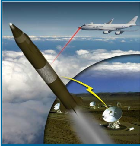
Temperature and Irradiance Sensor Matrix (TISM) – Direct measurement of laser irradiance and target temperature; AEGis is designing and testing the sensor mesh.
